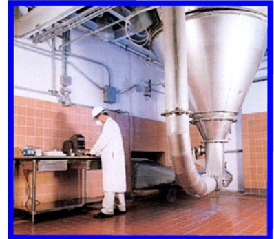
Dryer #4 with baghouse, transfer station and bulk 50,000 gallon tanks
